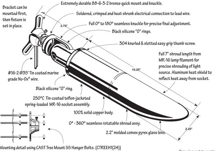
Mounting detail using CAST Tree Mount SS Hanger Bolts. (CTREEH1(24)) Note that bolts allow for breathing space between bracket and tree to prevent tree rot
