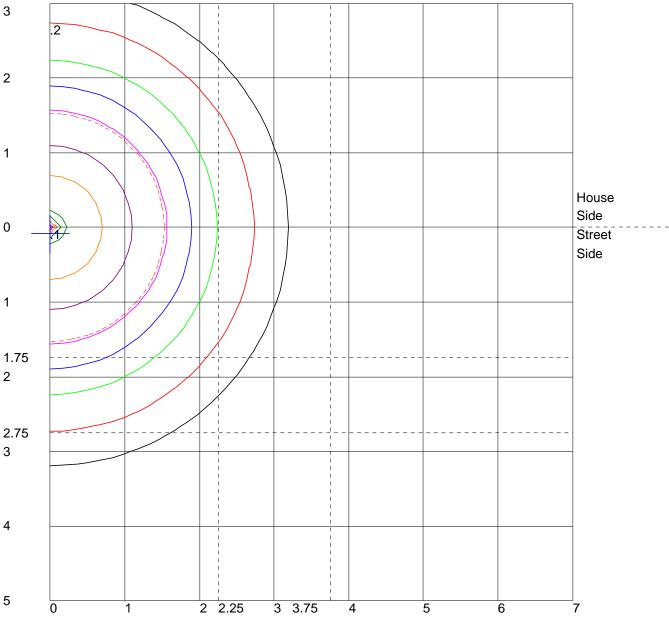
Distance In Units Of Mounting Height Values Based On 1.33 Foot Mounting Height 1/2 Maximum Candela Trace Shown As Dashed Curve
