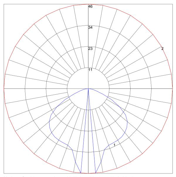
Maximum Candela = 45.99 Located At Horizontal Angle = 0, Vertical Angle = 5 # 1 - Vertical Plane Through Horizontal Angles (0 - 180) (Through Max. Cd.) # 2 - Horizontal Cone Through Vertical Angle (5) (Through Max. Cd.)
