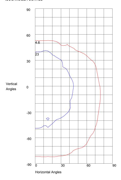
Maximum Candela = 46 Located At Horizontal Angle =-1, Vertical Angle = 5 50% Maximum Candela = 23 10% Maximum Candela = 4.6
