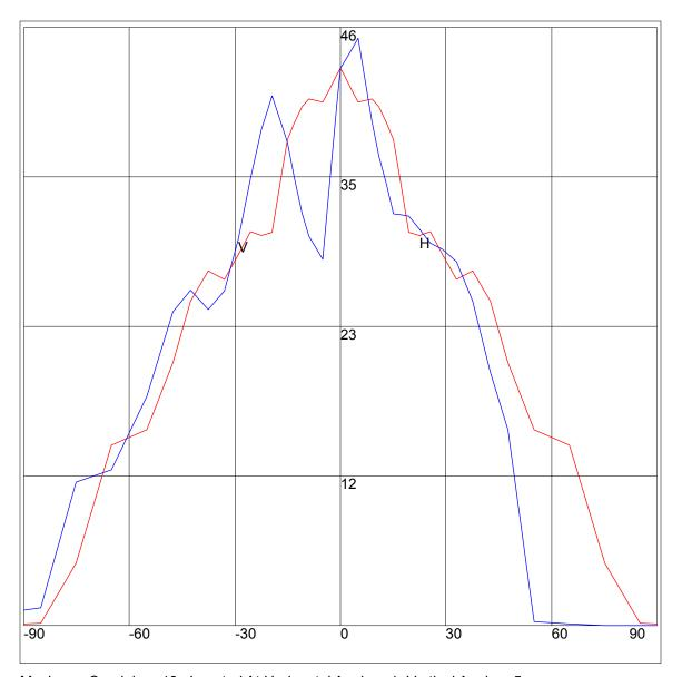
Maximum Candela = 46 Located At Horizontal Angle =-1, Vertical Angle = 5 H - Horizontal Axial Candela
