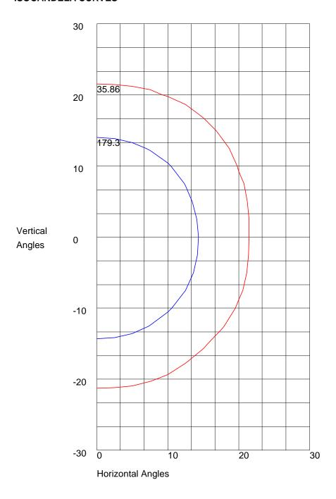
Maximum Candela = 358.6 Located At Horizontal Angle = 0, Vertical Angle =-5 50% Maximum Candela = 179.3 10% Maximum Candela = 35.86
