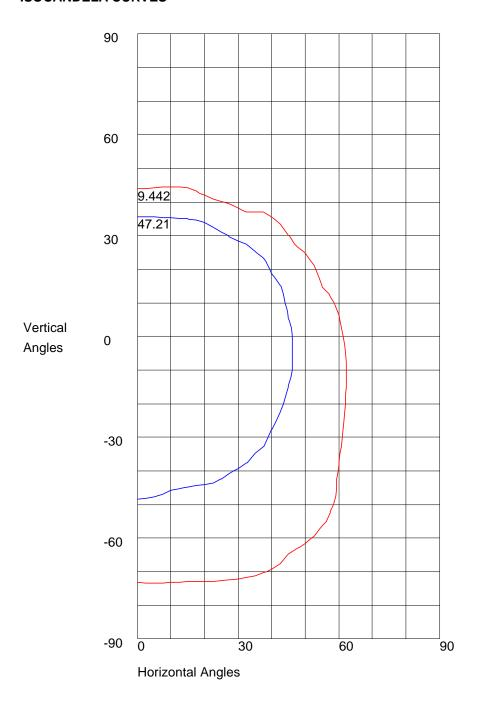
Maximum Candela = 94.42 Located At Horizontal Angle =-3, Vertical Angle =-3 50% Maximum Candela = 47.21 10% Maximum Candela = 9.442
