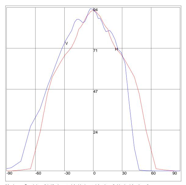
Maximum Candela = 94.42 Located At Horizontal Angle =-3, Vertical Angle =-3
