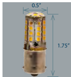
SLSCB250L Single Contact Bayonet LED; 2.5 Watts, 9 - 20 Volt operating range; 250 Lumen, Color Temp. 2750°K; IP67 Rated, 25,000 Hrs.
