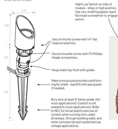
Product equipped with LED module. Module is screwed to fixture base. Optical lenses can be replaced by removing screws in lens retaining ring. Full instructions included in fixture box.
