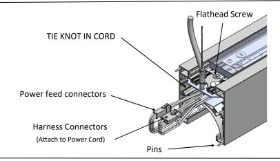
For row mounting fixtures attach male end of harness to female end of harness and slide fixtures together until no gap remains.
