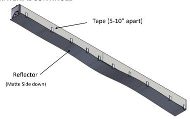
Push Reflector upward and remove tape
