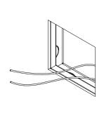
Wall thickness shall not exceed 1/2" (13mm)
