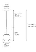
Light distribution \_\_\_\_\_ Diffused Luminaire weight 3.45 lbs / 1.57 kg
