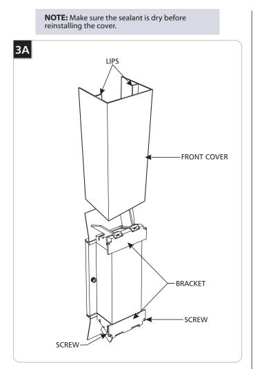
1 Carefully slide the front cover onto the fixture ensuring that the lips are behind the brackets and rest on the screws.
