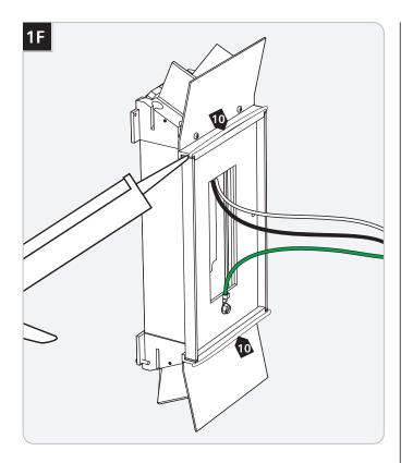
**For wet locations**, apply caulk **only** along the top and bottom of the fixture base with waterproof construction sealant.
