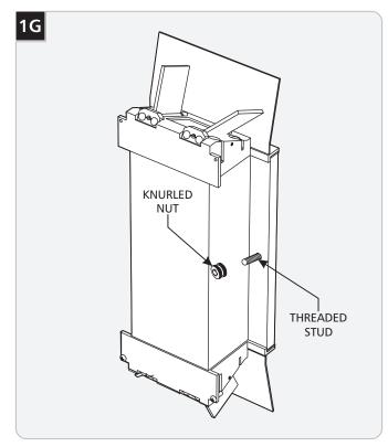
Neatly tuck all wires and wire nut connections into the electrical box, mount the fixture onto the threaded studs, and secure it in place by screwing the knurled nuts onto the studs.
