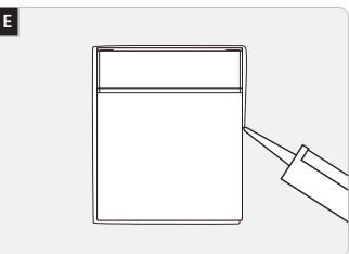
**For wet locations**, caulk around the base with waterproof construction sealant.
