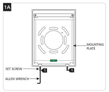
With the Allen wrench provided, back out (do not fully remove) the set screws at the base of the fixture.
