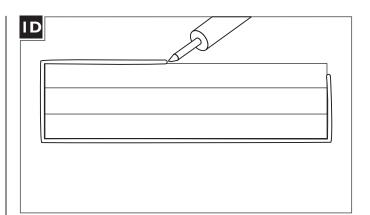
**8** For wet locations, caulk around the base with waterproof construction sealant.
