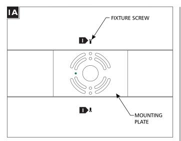
Remove the two fixture screws located on the top and bottom of the fixture base.
