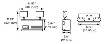
Meets Life Safety Code illumination standard; average of 1.0 FC, no point less than 0.1 FC, max to min ratio of 40:1. Assumes open space with no obstructions, mounting height: 7.5' and reflectances: 80/50/20. Analysis based on independently tested photometrics.
