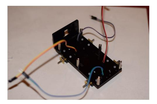
6) Attach, the Male 2 Female jumper wires to the motors.
