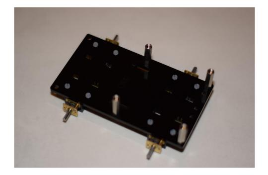
3) Add the four of the pillars using the short 3mm screws
