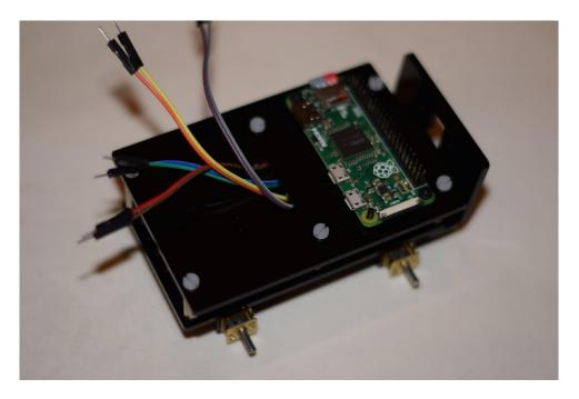
7) Feed the jumpers through the hole in the middle of the top plate and use the 6 x 3mm screws to fix the top plate.
