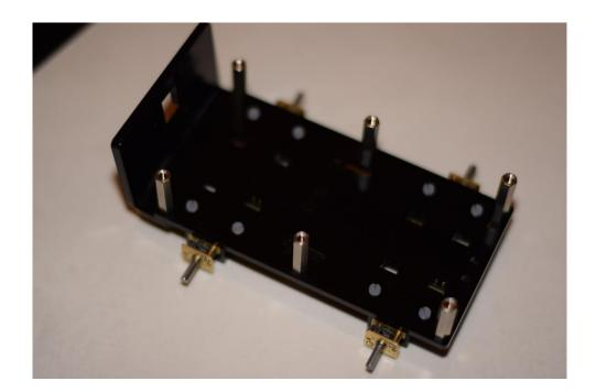
4) Fix the camera plate to the front of the with the long 3mm screws and the last pillars
