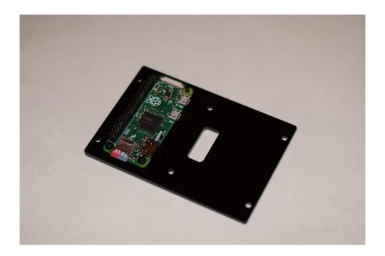
5) Attach your Raspberry Pi using 4 x 2.5mm screws and 8 nuts, using 4 nuts to space the Pi off the plate. The remaining nuts to secure the Raspberry Pi.
