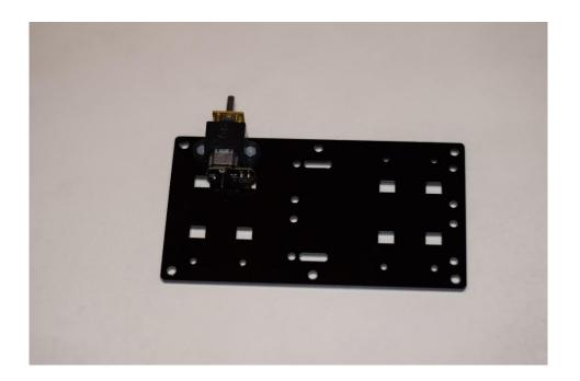
1) Attach the motor to the bottom plate, with the motor bracket and 2.5mm metal screws. The head of the pirate should be towards the closest edge.
