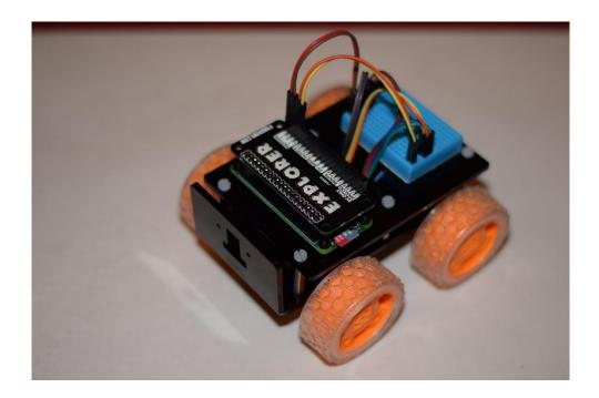
10) Attach the wheels, line up the flat section on the motor shaft with the one on the wheel, then push to fit.
