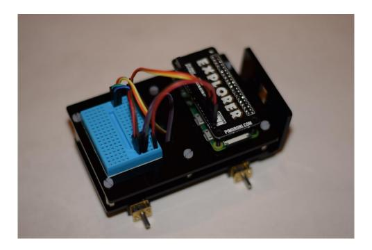
8) Fit the bread board to the top plate and plug in the headers from the motors, the pins go across 2 columns for each side.
