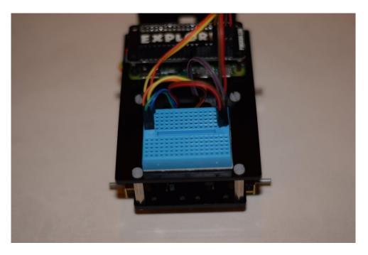
9) Attach the Explorer pHat to the Raspberry Pi, then the male 2 male jumpers between bread board and the Explorer pHat.
