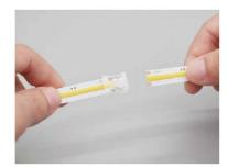
Insert each end of led strips into the end of the connection terminal respectively, make sure the metal clip is in same side as the metal solder pad of led strip.
