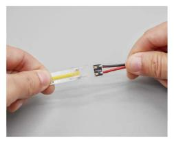
Insert one end of led strip and wire connector into both ends of the connection terminal respectively to ensure that the metal clip is on the same side as the metal solder pad of led strip.
