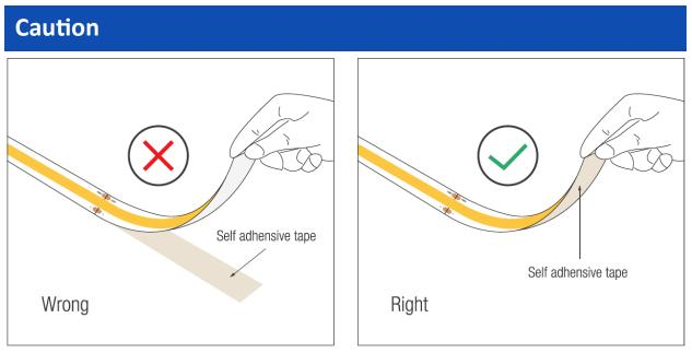
If the led strip needs to be torn upwards, please make sure that the self adhesive tape is torn with the led strip, else the led strip would be damaged.
