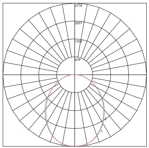
Maximum Candela = 2715.561 Located At Horizontal Angle = 0, Vertical Angle = 0 #1 - Vertical Plane Through Horizontal Angles (0 - 180) #2 - Vertical Plane Through Horizontal Angles (90 - 270)
