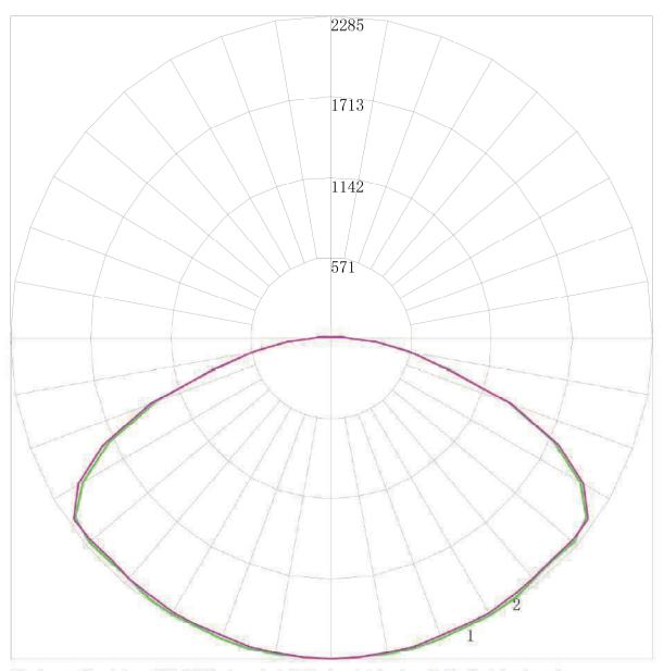
Maximum Candela = 2284.574 Located At Horizontal Angle = 0, Vertical Angle = 0 # 1 - Vertical Plane Through Horizontal Angles (0 - 180)
