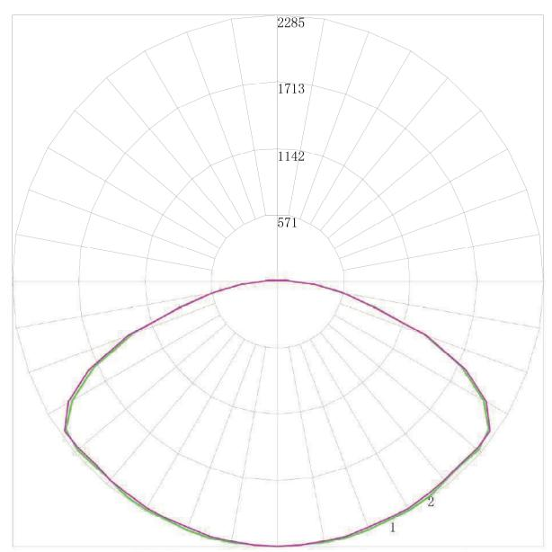
Maximum Candela = 2284.574 Located At Horizontal Angle = 0, Vertical Angle = 0 # 1 - Vertical Plane Through Horizontal Angles (0 - 180) # 2 - Vertical Plane Through Horizontal Angles (90 - 270)
