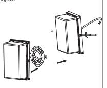
**Step 6**: Screw and fasten the PC frame back to the light with one screw on the top and two screws at the bottom.
