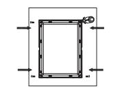
Step 4: Screw and fasten the PC frame back to the light with one screw on the top and two screws at the bottom.
