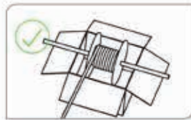
Slide a spindle into the roll and then place the roll with spindle on top of the box provided.
