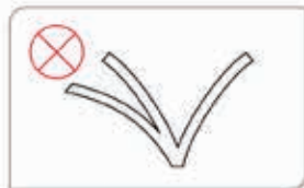
Do not repeatedly bending This will damage the circuit
