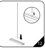
12. The bottom of the assembled pole slides into the round socket in the centre of the base unit.
