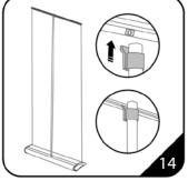
14.The hook at the top of the pole slips into the rear slot of the banner beam. A marker on the beam indicates the beam's centre where the pole should be inserted.
