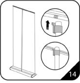
14.The hook at the top of the pole slips into the rear slot of the banner beam. A marker on the beam indicates the beam's centre where the pole should be inserted.
