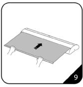
Carefully allow the graphic to recoil into the base unit (it may be useful to have an assistant hold the base steady)
