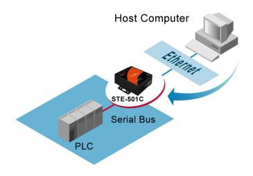
**TCP Client Mode :** STE-501C can be configured as a TCP client on TCP/IP Network to establish a connection with other applications (server) in host computer actively. After the connection is established, data can be transmitted between serial device and host computer in both directions.
