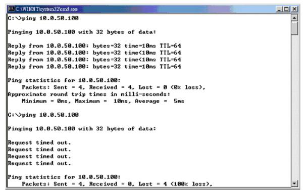
Figure 7.1 Standard TCP/IP utility ping command
