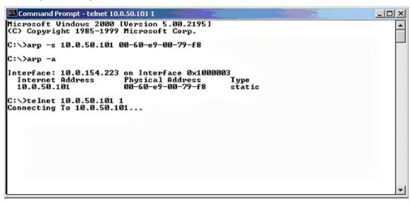
Figure 3.27. Assigning a new IP address by ARP command
