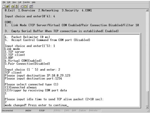
Figure 3.11 Link Mode-TCP client setup
