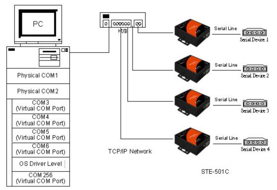
Figure 4.1 Virtual Com connection diagram
