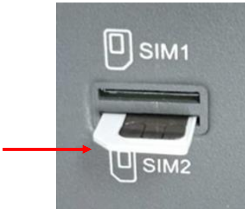
SIM2: Exposed card side up, notch is facing to the left.
