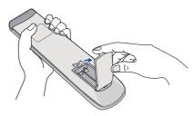
② Align and insert two AAA batteries according to their plus and minus ports (as indicated in the remote control).
