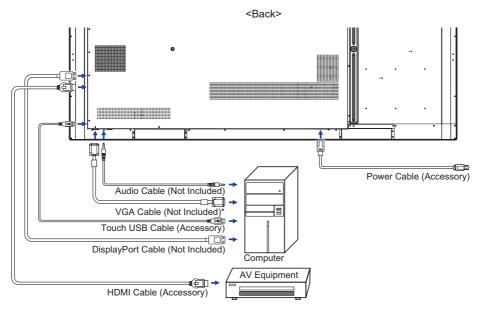
\* VGA cable is not supplied with the monitor. If you use low quality VGA cable, it may cause a result of electro-magnetic interference. Please contact the ijyama Support Centre in your country if you wish to connect the monitor via the VGA input.
