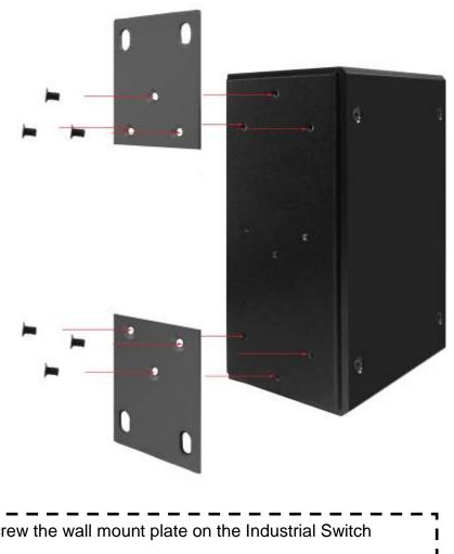
Screw the wall mount plate on the Industrial Switch
