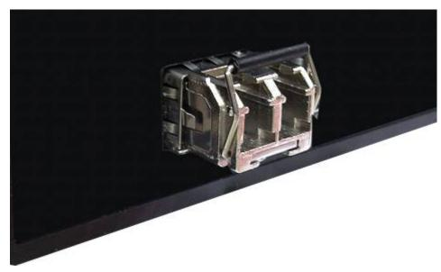
Figure 2.9: Transceiver Inserted
