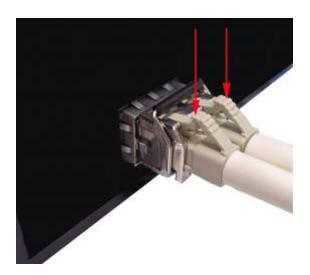
Figure 2.11: Remove LC connector
