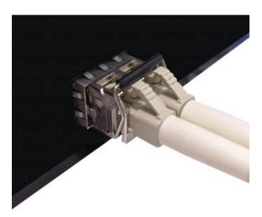
Figure 2.10: LC connector to the transceiver
