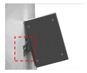
2. Then, lightly push the DIN-Rail into the track.
