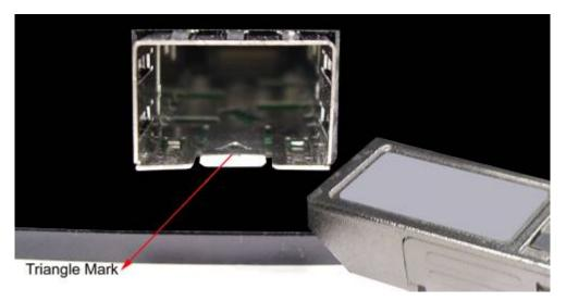
Figure 2.8: Transceiver to the SFP module
