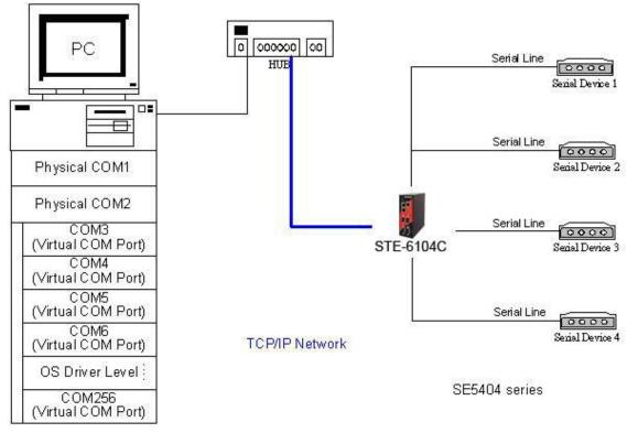
Figure 4.1 Virtual Com connection diagram
