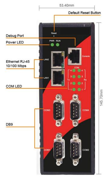
Figure 2.1 Front Panel Interfaces
