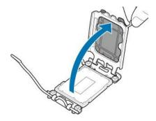
3. Align and seat the processor package on the socket. Make sure the gold arrow is located in the right direction.
