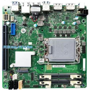
Simply find the appropriate slot for your add-in card and insert the card firmly. Do not force any add-in cards into any slots if they do not seat in place. It is better to try another slot or return the faulty card rather than damaging both the motherboard and the add-in card.
