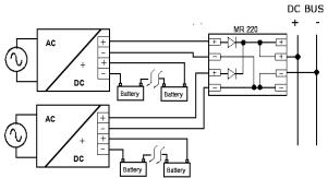
Parallel connection "Redundancy"
