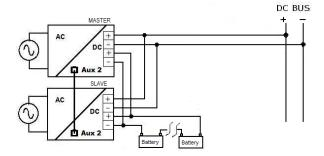
Power supply can be paralleled to increase the output power, devices can be paralleled for 1+1=2 to obtain the double power of a single unit. Only SIZE 3 devices can be connecter in parallel to attain the sum of the current at the same output voltage. It is necessary to use a standard UTP or order Cable code: RJCONN45 for RJ45, and connect to Aux2 of each device. The communication protocol is based on CAN2.0A standard.
