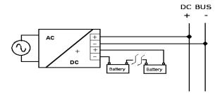
Typical application for All In One device, one output for Load "DC Bus", one Input / Output for connection to the battery.
