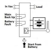
Input: Single-phase 115 – 277 Vac Output Load: power supply 24 Vdc; 3 A Output Battery: charging 24 Vdc; 3 A
