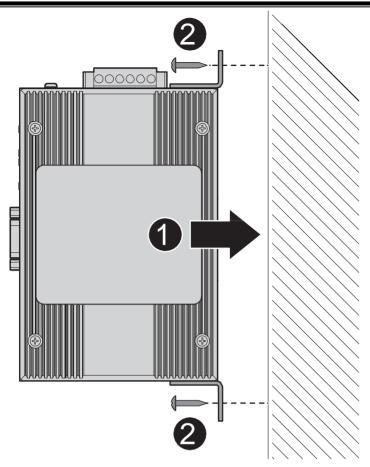
Figure 3.5 Wall Mount Installation
