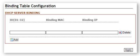
Figure 5.68 – DHCP Server Binding Interface
