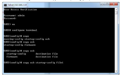
Fill in the folder and filename behind the "copy usb startup-config" command.
