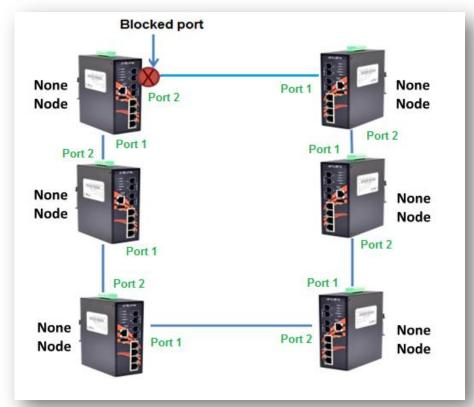
Figure 5.27 – Non-Configured Architecture
