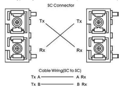
Figure 2.6 - Fiber Ports Connection
