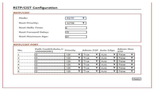
Figure 5.30 – RSTP Configuration Interface
