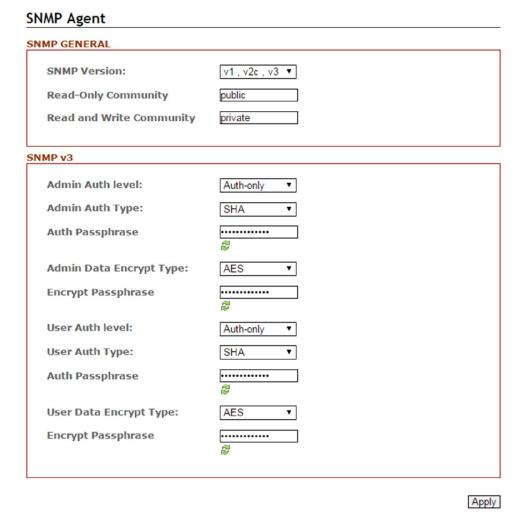
Figure 5.56 - SNMP Agent Setup Interface
