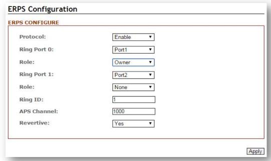
Figure 5.24 - RPL Owner Node Setup Example
