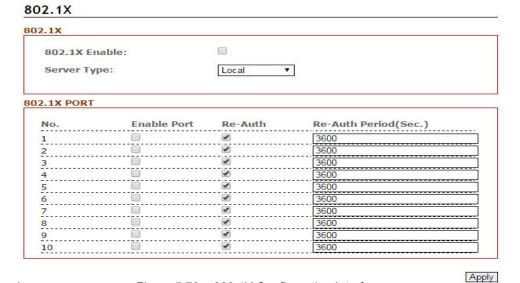
Figure 5.73 - 802.1X Configuration Interface
