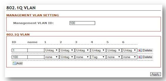
Figure 5.40 - 802.1Q VLAN Settings Interface
