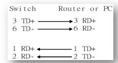
Figure 2.4 Straight-Through Cable Schematic
