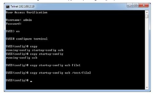
Fill in the folder and filename behind the "copy startup-config usb" command.
