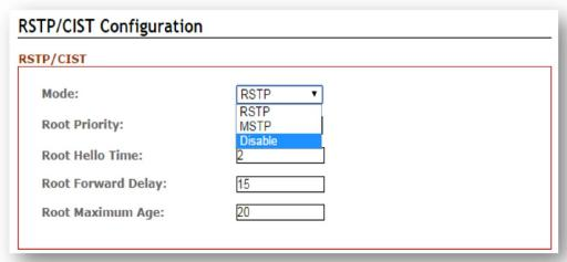
Figure 5.21 – RSTP/CIST Configuration Interface
