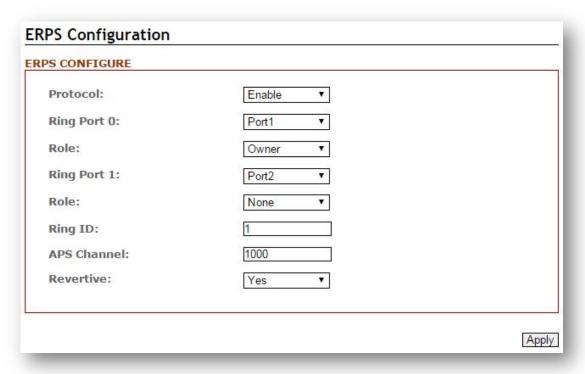
Figure 5.18 – ERPS Configuration Interface
