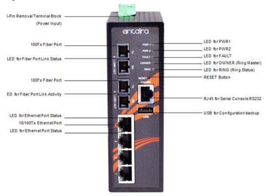
Figure 2.2 - The Front Panel of LMX-0602 Series
