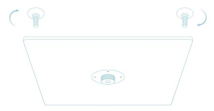
1. Turn Base plate upside down) and screw 4 feet into the threaded holes in each corner. (feet are optional but allow clear passage for dirt, leaves and water to move under your stand reducing damage and exposure to elements).
