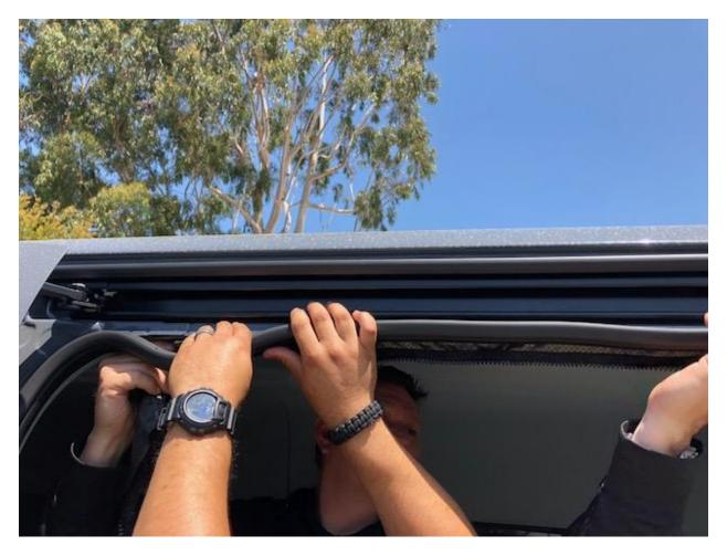
5) With the top of the bug net frame in place you can now slowly remove the rubber gasket working your way down the left side of the slider door opening.
