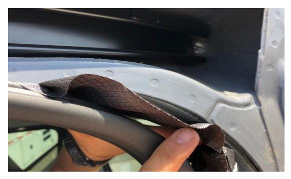
4) Taking your time, work your way from the right to the left securing the top of the frame of the bug net to the slider door opening.
