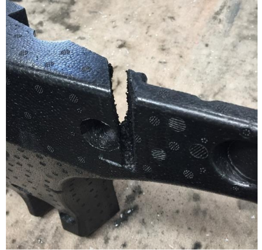
Cut the foam with a knife poke out with a screw driver
