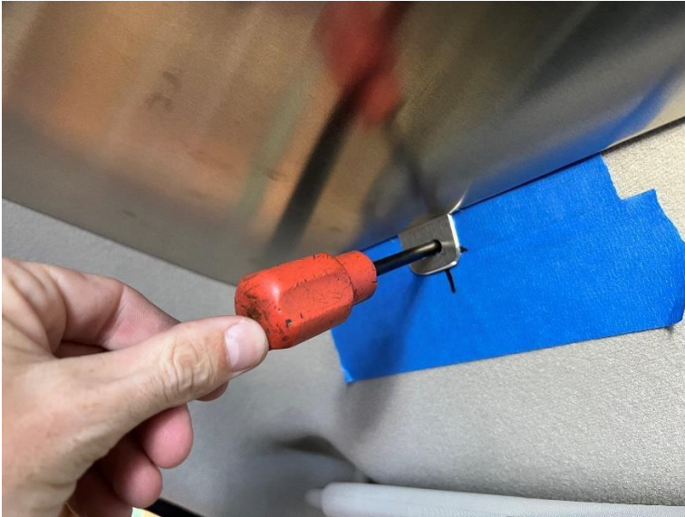
Find the Mounting Bracket Hole/Threads, Behind the headliner.
