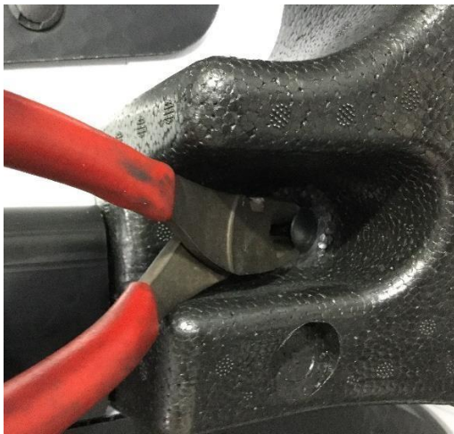
Cut Head Off Rivet
