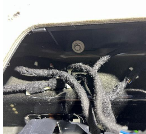
Remove Bolt inside Light Housing
