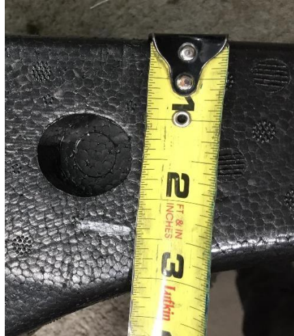
Mark about 2-1/2" to Cut down
