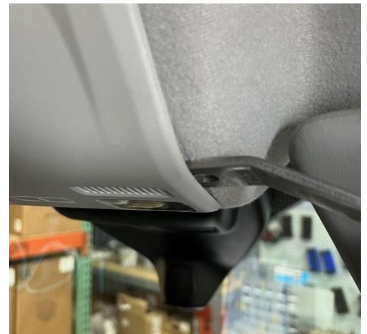
Push Tab With Flathead Screw Driver
