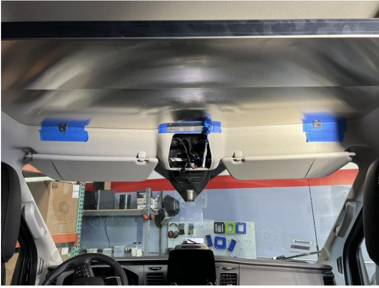
Hold Up Shelf into place and set on Rear Mounts
