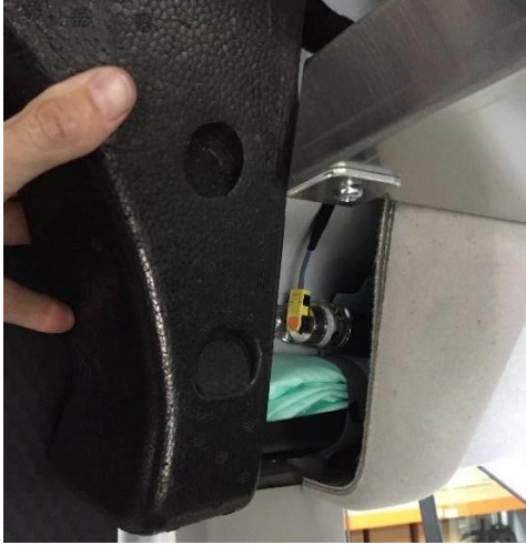
Press the Foam into the bracket so it leaves an indentation
