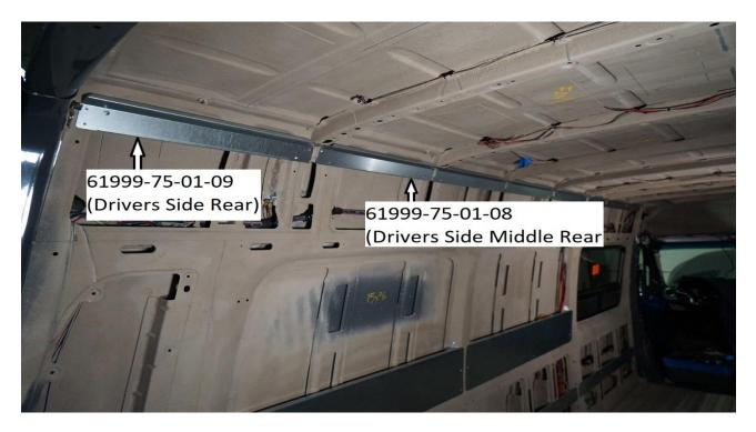
\*\*\*NOTE\*\*\* Picture shown below is referencing a 170 EXT Model. In the 170 models the rear brace used is #61999-75-01-1 (smaller size than shown in 170 EXT Model) in place of #61999-75-01-06
