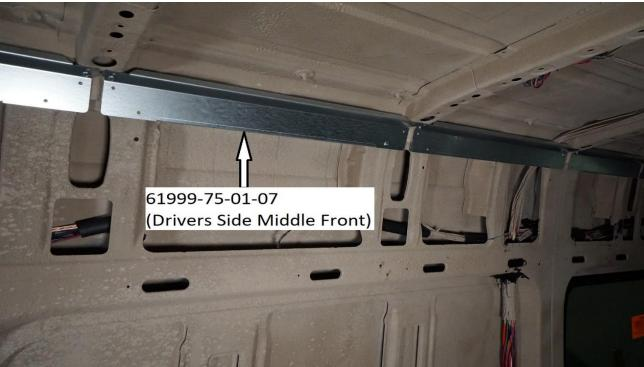
\*\*\*NOTE\*\*\* Picture shown below is referencing a 170 EXT Model. In the 170 models the rear brace used is #61999-75-01-11 (smaller size than shown in 170 EXT Model) in place of #61999-75-01-09
