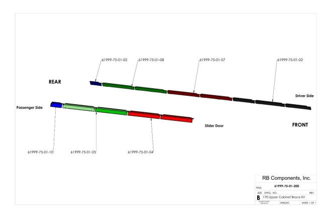
2) Once the individual braces have been identified we suggest aligning them properly. Each brace has a cut out for clearance on a small bump out in the frames interior. Align the driver and passenger side braces to align with these cut outs. Once aligned the brace is held up to the top and side support structure of the van. Using a #11 drill bit drill thru the holes and rivet braces into place as shown.
