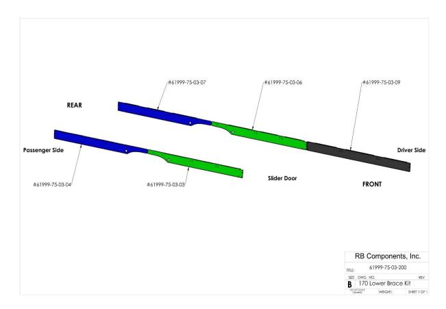
2) Once the individual braces have been identified we suggest aligning them properly. Each brace has a cut out for clearance on a small bump out in the frames interior. Align the driver and passenger side braces to align with these cut outs. Once aligned the brace is held up to the top and side support structure of the van. Using a #11 drill bit drill thru the holes and rivet braces into place as shown.
