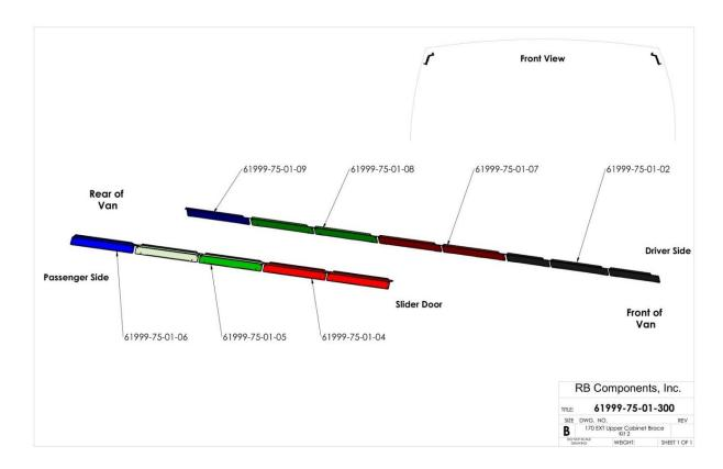
2) Once the individual braces have been identified we suggest aligning them properly. Each brace has a cut out for clearance on a small bump out in the frames interior. Align the driver and passenger side braces to align with these cut outs. Once aligned the brace is held up to the top and side support structure of the van. Using a #11 drill bit drill thru the holes and rivet braces into place as shown.
