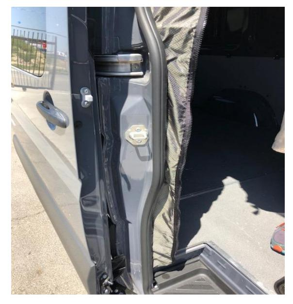
8) With the frame in place we can now zip the screen to the frame. First start by zipping the very top portion of the screen to the upper portion of the bug net frame as shown.
