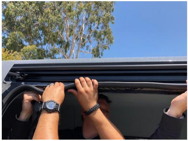
5) With the top of the bug net frame in place you can now slowly remove the rubber gasket working your way down the left side of the slider door opening.
