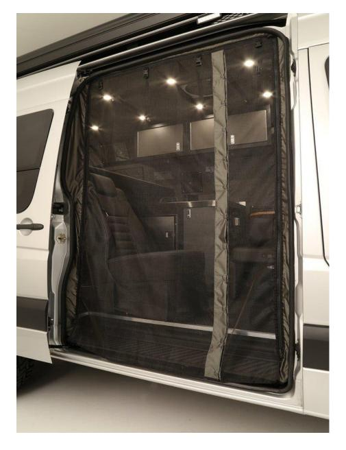
10) The bug net screen can be accessed a few different ways. Either by the center pass through (*magnetic self-closing buttons*) or by unzipping the sides.
