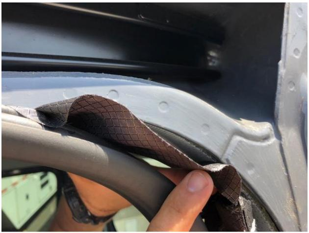
4) Taking your time, work your way from the right to the left securing the top of the frame of the bug net to the slider door opening.
