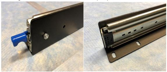
4) With slide rails mounted the next step is mounting the aluminum tray/tray rails (for DIY Kit) to the slides. To do this you will need to fully extend each slide and line up the mounting holes in the tray with the corresponding holes in each slide using the #10-24 x ½" Phillips head screws and #10-24 locknuts.
