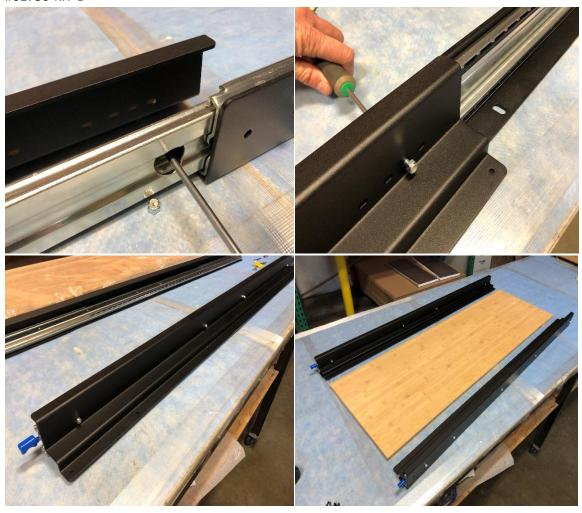
2. With DIY tray rails now mounted to the slide assembly the next step is to find out where you are mounting it and determine the width of the wood that is needed to complete the tray bottom. This is done by installing the left and right assemblies in location and measure across to determine the width of wood needed.
