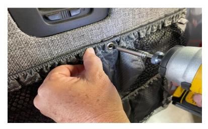
6) The lower part of the stuff bag does not have a steel grommet. In this area we place the self drilling screw in the lower area of the bag as shown.
