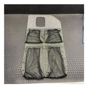
4) With the stuff bag fully slipped onto the lower rear door panel you can now mount it back onto the rear door of your van. Line up the lower rear door panel on your door. Start by screwing in one of the upper corners using the self drilling screws that are provided. Once the upper screws have been installed we can secure the lower part of the panel and stuff bag.
