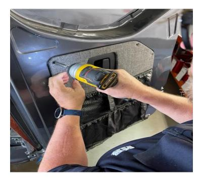
5) Secure the middle part of the bag by securing a screw thru the steel grommet as shown.
