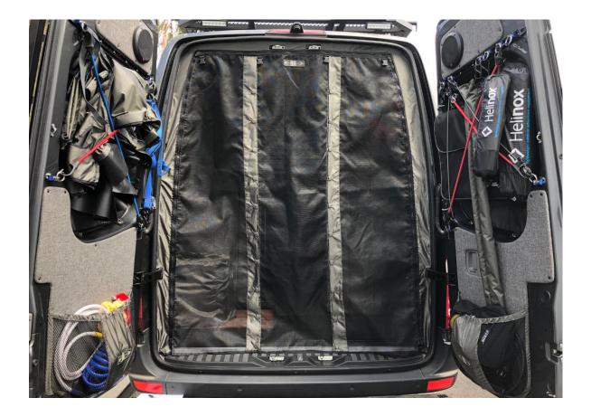
9) The bug net screen can be accessed a few different ways. Either by the center pass through (*magnetic self-closing buttons)* or by unzipping the sides.
