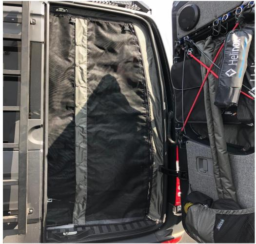
11) The rear door bug net does not need to be removed or rolled up to have the rear doors closed.
