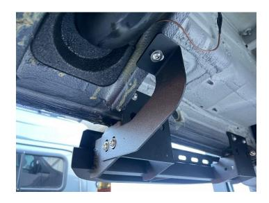
3) Next is to locate and install the passenger side long entry step. The mounting process is the same as the driver side step. Before mounting the support braces its best to first mount the step to the weld seam of the van to ensure it is
