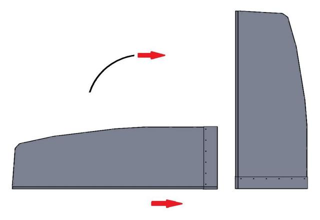
Rotate the shower with the shower face down. The easiest way to bring the shower into the van is from the rear of the van. Once the shower inside the van you can then tilt the shower upwards.
