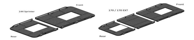
2) Flip racks over. Using 3/16'' all wrench and 1/2'' socket, bolt the racks together as shown using the  $5/16-18 \times 1/2''$  button head cap screws, 1/2'' uss flat washers and 1/2' locknuts. For 1/2 & 1/2 EXT racks, repeat this assembly for the rear rack.
