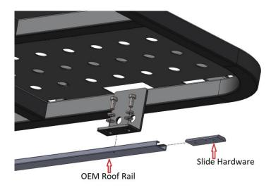
4) For 144 Roof racks this completes the installation. For 170 / 170 EXT roof racks you will need to unpack and repeat the installation for the rear rack. If your van has one or no roof vents a roof vent cover is sold seperately (#70000-151-B). This cover aligns with the top panel and is drilled and riveted into place (mounting hardware provided) giving your rack that full finished look.
