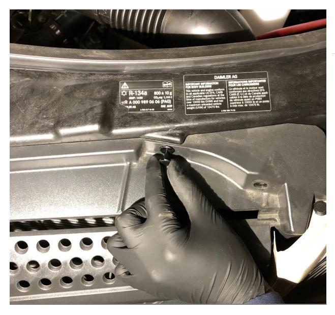
2) Once the screws and snap buttons are removed from the upper part of the grill pull the top part of the grill back slightly to access the lower retaining clips.
