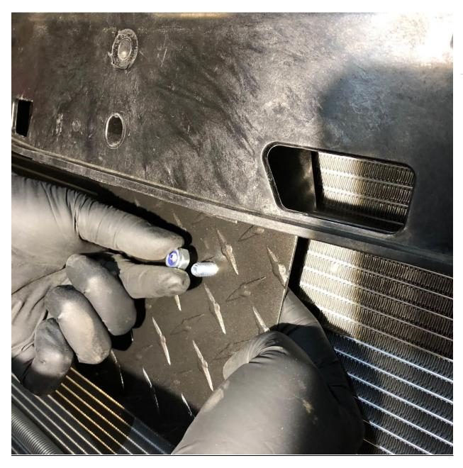
7) Place the horn over the nut. This will keep the nut in place allowing you to tighten the bolt from the backside of the horn mounting bracket. Using a 13mm open end wrench tighten the horn to the mounting bracket as shown.
