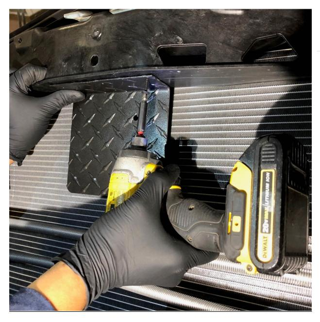
6) With the horn mounting bracket in place take the nut and bolt that came with the horn. This will be used to mount the horn to the mounting bracket. Take the bolt and insert it through the back side of the bracket as shown. Next thread on the nut a few turns.
