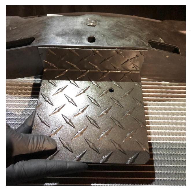
5) With the bracket centered, use the (6 pcs.) #8 x  $\frac{3}{4}$ " self tapping screws to secure the bracket to the underside as shown (making sure to not overtighten).
