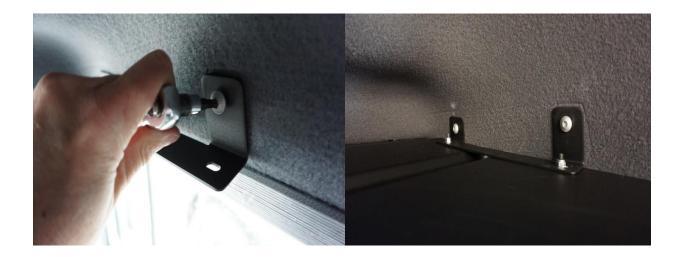
4) With the forward mounting brackets installed next will be installing the rear mounting brackets using the #20 torx wrench. To not tighten these brackets just yet as they should be able to spin out of the way. This will make it easier when the headliner shelf is lifted into place.
