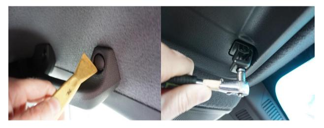
2) Remove the plastic clothes hanger as shown. Using a #20 torx wrench to remove this screw. Because the headliner is a tight fit to the sides of the van, we recommend using tape along the top part of the plastic as this will protect the plastic trim during installation.
