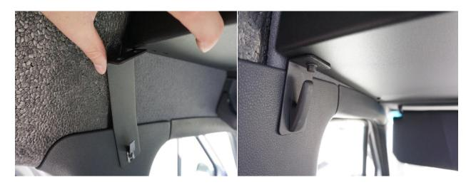
7) With the hardware provided secure all the bolts with the nuts on top of the headliner shelf as shown using a 10 mm socket and open end wrench to tighten headliner to the brackets.
