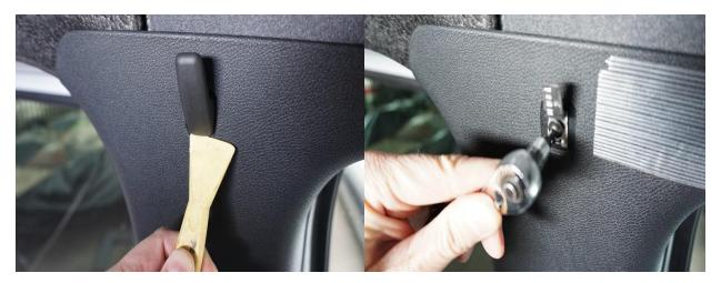
3) Install the Left and Right Forward brackets using a #30 torx wrench. Making sure that the raised part of the bracket is facing towards the rear of the van as shown.
