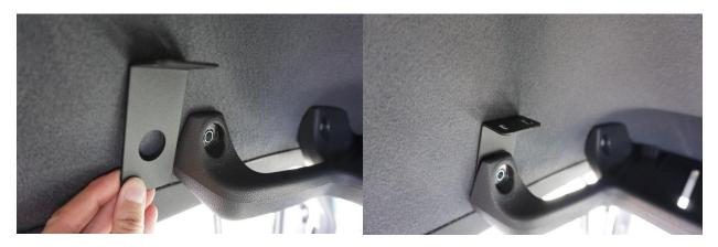
3) Before installing the headliner swing back the rear mounting bracket. This will make it easier when the headliner is put in place.
