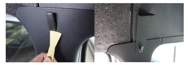
2) Using a #30 Torx wrench remove the bolt in the back of the plastic handle. Place the smaller front bracket behind the plastic factory grab handle as shown. Thread the bolt into place but do not tighten at this time. Do this to both sides.
