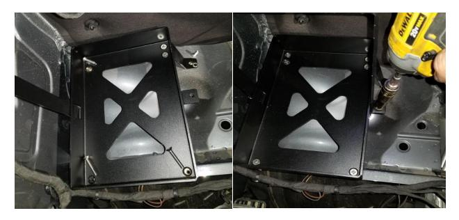
7) With the passenger side battery tray installed the driver side tray mounts exactly the same way. But first you will need to unclip the silver ECU unit from the housing and remove the plastic mounting tray using a 10mm socket wrench.
