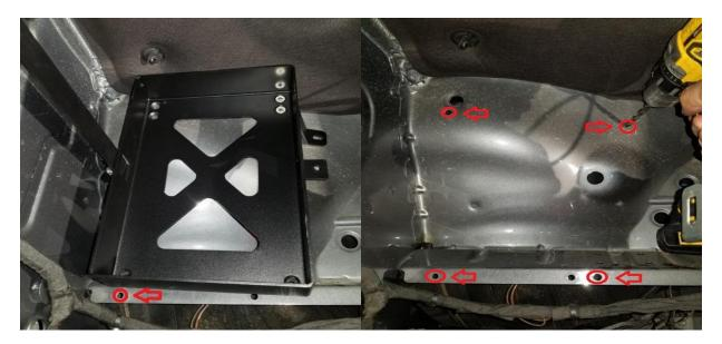
5) Insert the 4 gold riv nuts into the tray mounting holes you just drilled and secure the riv nuts in place using the riv nut fastening tool.
