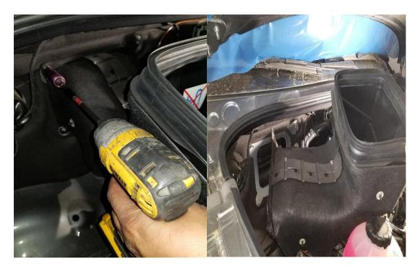
2) With the air box removed you will need to build up the passenger side battery tray as shown. Please take note that when building the tray to use the rear support bracket <u>WITHOUT</u> the hole as shown. Do not tighten straight bracket completely. Leave about ¼" gap so when the batter is installed the top strap will align to be tightened down holding the battery in place.
