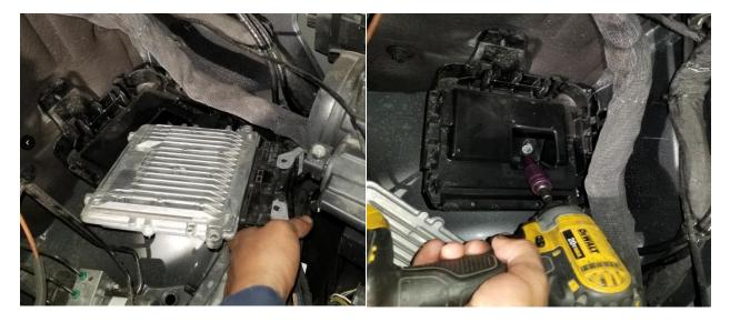
8) The lower mounting bolt will need to be cut so it clears the battery tray.
