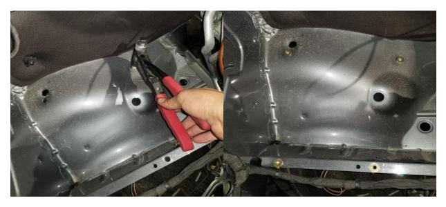
6) Mount battery tray in location using the hardware provided.
