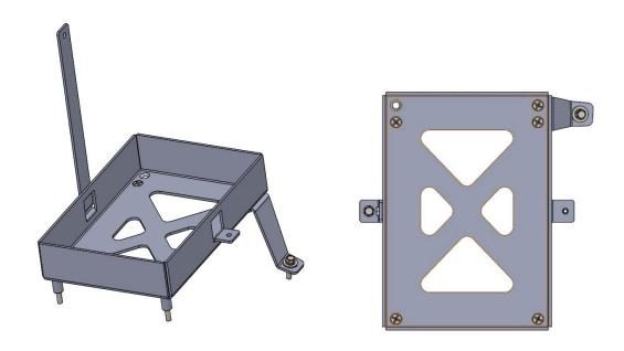
3) Before placing the battery tray in location the zip ties holding the wiring to the front wall will need to be removed. The front of the battery tray will sit on this front wall.
