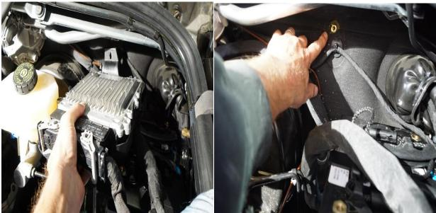
13) With ECU riv nut installed use the (# 60951-710)1/4-20 x 1-1/4 Hex head with (#60951-675) washer to secure ECU to bulkhead wall. Note: the bottom of the plastic mounting tray should be resting on top of the battery tray. This will help support the weight of the ECU.
